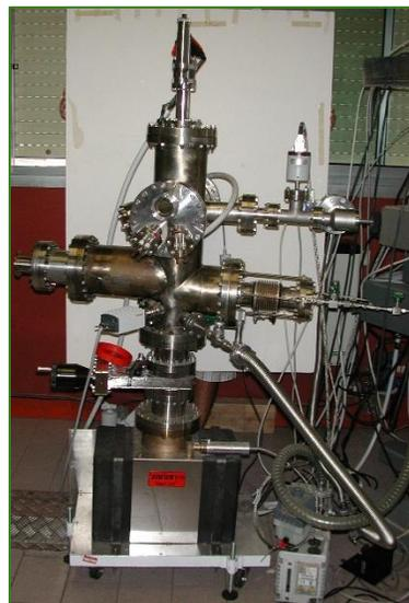
A system for the chemical vapor deposition growth of carbon nanostructures: carbon nanotubes (CNT) films or sponges, spheres
